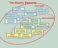
confused, the Smart Grid is not smart metering – the smart grid is a much broader set of technologies and solutions (see diagram).
